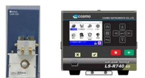
LS-R740SS performs highly sensitive leak test on micro volume parts. The part to be tested is set on a fixture, and inside of the part is pressurized to measure the pressure change generated by leak.
